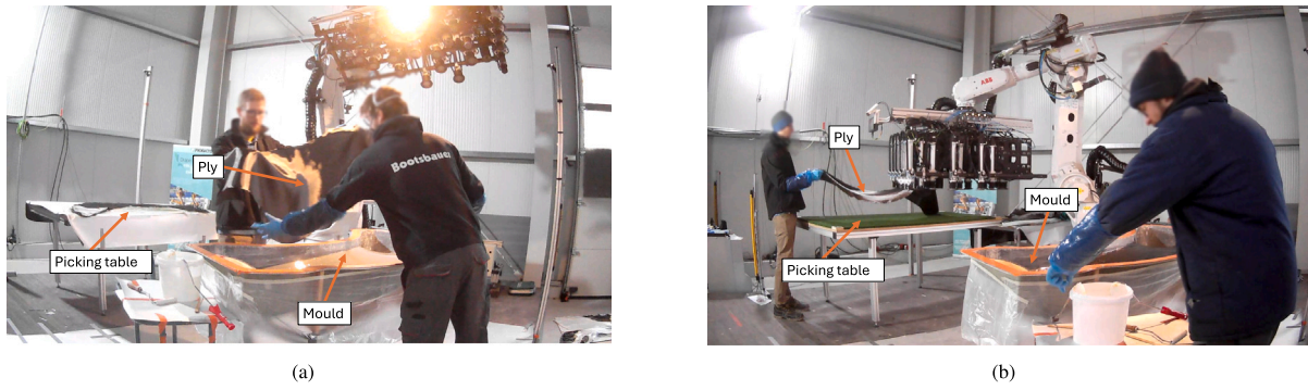
Fig. 16. Production of a boat propeller (UC3): (a) reports one operator while making the manual transport of the ply from the picking table to the mould with the second operator giving support for the final placement in the mould and the impregnation, (b) reports the human–robot collaborative transport of the ply from the picking table to the mould performed by a single operator, while the second is waiting for the impregnation of the ply.
